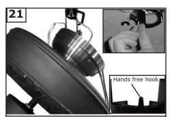
Remove the all thread studs from the lower part of the mounting bracket. Hang fan from mounting bracket by the hands free hook into a closed hole on the edge of the Canopy. Note: For Canadian mounting refer to Step #8.
